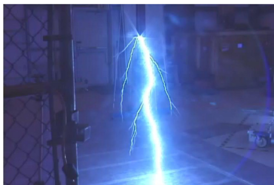
Fig. 5.10. Image of a 1.5 m spark in air generated by a 1.5 MV Marx generator for which it was discovered that long laboratory spark in air produces X-rays similar to lightning [182].
